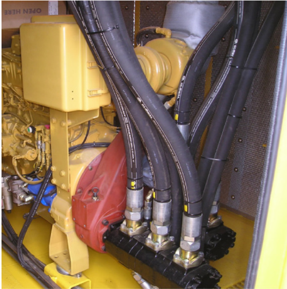
Platform Support Fixed Gear Type Hydraulic System
