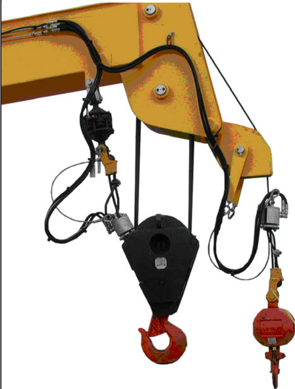
Mechanical Anti-Two-Block System Simple Seatrax arrangement for use on high use floating cranes.
