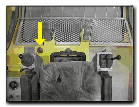
The emergency hoist brake foot button is located on the left-hand side of the cab floor and is redundant to the fail-safe features of the Seatrax spring-applied, external contracting band drum brakes.
