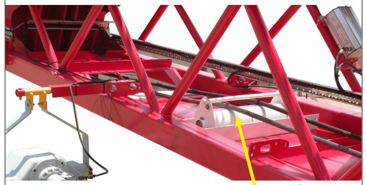
To provide increased boom protection, Seatrax engineers have developed the new boom tip rollers, a solution that not only shields the boom and wire rope from damage but also makes crane operation easier.
