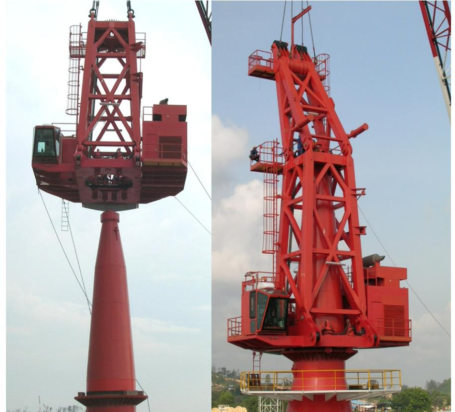
All Seatrax cranes are based on the well-proven kingpost concept. This basic design consists of a stationary or fixed kingpost and a revolving superstructure, which fits over and revolves around the stationary post.
