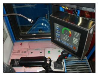
The Seatrax CCM14000 simplifies the monitoring of primary and auxiliary crane systems, including hydraulic systems, hoists and prime mover. It incorporates a hard wired network of boom angle and hoist load cell sensors that communicate with the display terminal.
